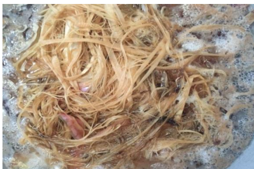
Figure 1 Alkali treated banana stem fiber
